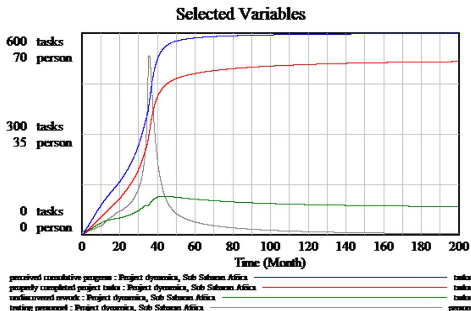
Fig. 10: Comparison of trends of perceived cumulative progress, properly completed project tasks, undiscovered rework and testing personnel
