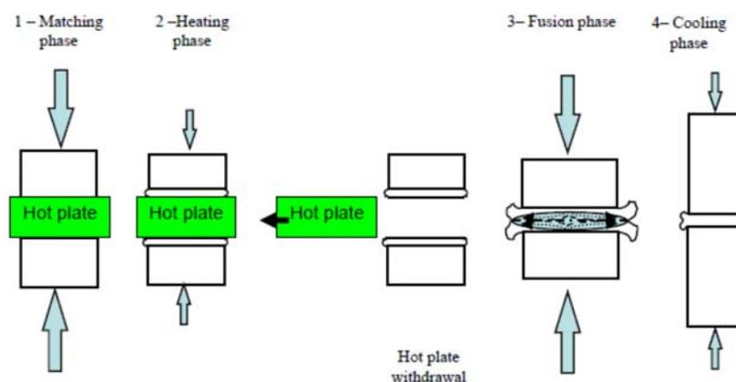
Figure 1: Hot plate welding process, Source: Hot Plate Welding (2006)
