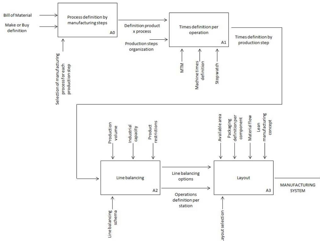
Figure 4: IDEF0 diagram proposed for a manufacturing system definition model
