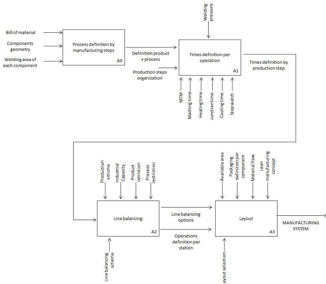
Figure 5: IDEF0 diagram proposed for a hot plate welding system
