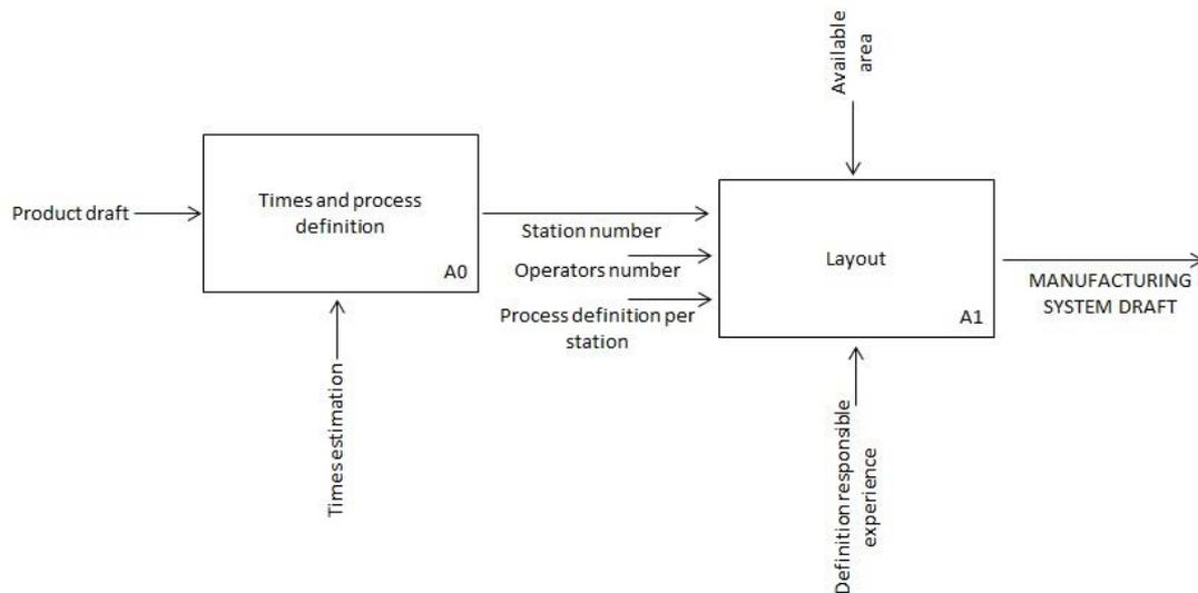
Figure 3: IDEF0 diagram representation of current manufacturing system scenario
