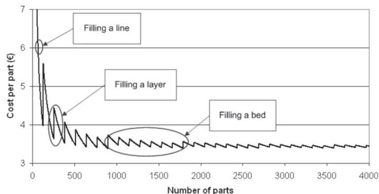
Fig. 3: Cost behaviour SLS production (Ruffo et al., 2006)
