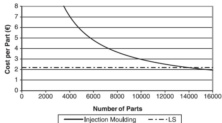
Fig. 2: Break-even analysis: Laser sintering, injection moulding (Ruffo et al., 2006)
