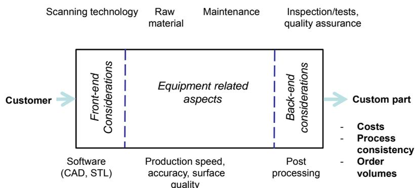
Fig. 6: Technology factors in the AM production creation process
